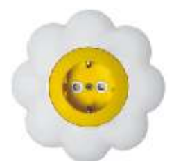
Two-pole socket-outlet with protection Flower (yellow / white) IEC 60884-1, CEE7 16A/250V; IP 20
